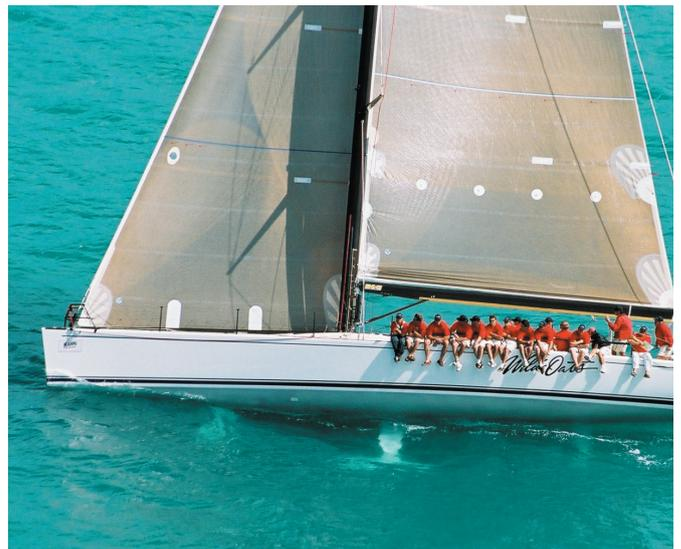
Gurit met the structural requirements of this design by specifying SE 84 carbon prepregs combined with Nomex cores throughout to achieve an all up structural weight of less than 2 tonnes and an all up sailing weight of just 11 tonnes. By combining experience in Open 60 class racing yachts and several large racers and racer cruisers, Gurit was able to design a fully composite canting keel structure that houses the entire keel mechanism without unduly obstructing the interior.
